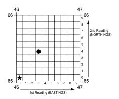
To give the six-figure grid reference, first of all identify the grid square, in this case 4665. The third figure obtained by dividing the space between grid lines 46 and 47 into ten equal parts. Similarly the sixth figure is obtained by a similar division of the gap between northings 65 and 66. This results in a grid reference of 463654 for the dot and 460650 for the star. It should be noted that the first tenth is 0 and the last tenth is 9 in the divided grid square.
